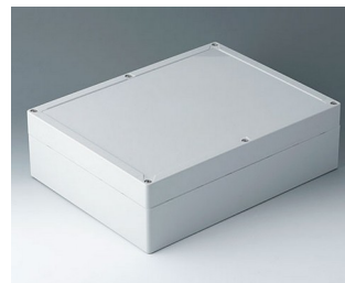
C7030101 IN-BOX ABS (UL 94 HB) light grey RAL 7035 302x232x90mm IP 66, IP 67, IK 07
