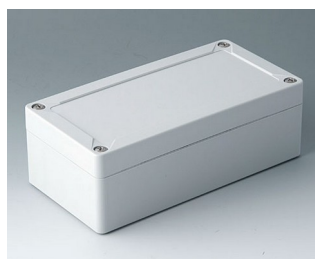
C7016011 IN-BOX ABS (UL 94 HB) light grey RAL 7035 162x82x55mm IP 66, IP 67, IK 07
