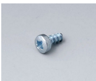
A0306031 Self-tapping screws 3 x 6 mm (PZ1)
