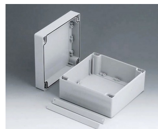
C2116162 ROBUST-BOX WIDTH 160, Vers. II PC (UL 94 HB) light grey RAL 7035 160x160x90mm IP 66
