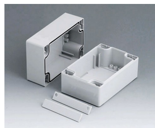
C2108122 ROBUST-BOX WIDTH 80, Vers. II PC (UL 94 HB) light grey RAL 7035 120x80x80mm IP 66
