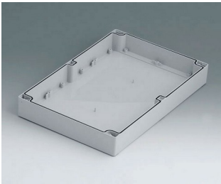
C2203001 Case shell 200, with groove ABS (UL 94 HB) light grey RAL 7035 300x200x40mm
