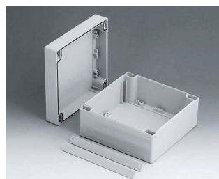
C2116161 ROBUST-BOX WIDTH 160, Vers. I ABS (UL 94 HB) light grey RAL 7035 160x160x90mm IP 66
