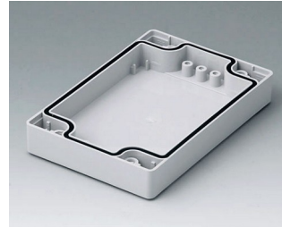
C0081201 Case shell 80, with groove ABS (UL 94 HB) light grey RAL 7035 120x80x20mm
