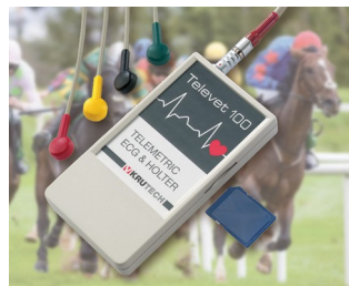
Telemetric ECG system for veterinary medicine
