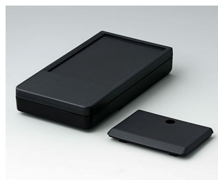
A9072209 DATEC-POCKET-BOX L PMMA (IR) (UL 94 HB) black RAL 9005 120x65x22mm IP 41
