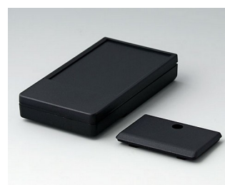
A9071219 DATEC-POCKET-BOX M PMMA (IR) (UL 94 HB) black RAL 9005 105x58x18,5mm IP 54
