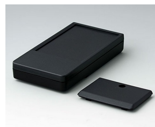
A9072119 DATEC-POCKET-BOX L ABS (UL 94 HB) black RAL 9005 120x65x22mm IP 54
