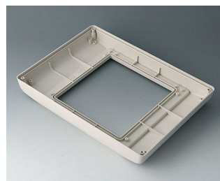
B4046757 Bottom part L high, version I ABS (UL 94 HB) off-white RAL 9002 275x195x36,5mm IP 54 opt.
