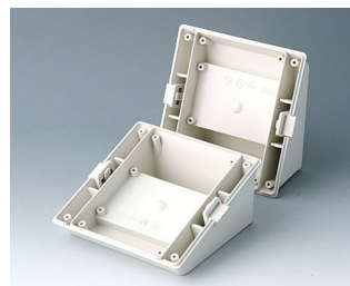
B4042847 Base S - desk-top/wall - ABS (UL 94 HB) off-white RAL 9002 123x123x53mm
