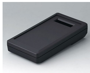
A9073319 DATEC-MOBIL-BOX S, Vers. III ABS (UL 94 HB) black RAL 9005 152x83x33,5mm IP 65 opt.
