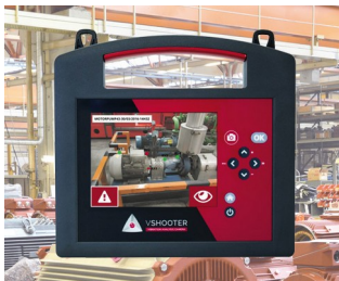
Diagnostic camera for illustrating the machine status
