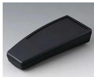
A9068119 SMART-CASE XL, Vers. II ABS (UL 94 HB) black RAL 9005 168x74,4x35,4mm IP 65 opt., IP 40
