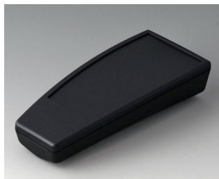
A9067219 SMART-CASE L, Vers. II PMMA (IR) (UL 94 HB) black RAL 9005 140x62,7x30,5mm IP 65 opt., IP 40
