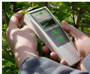
Chlorophyll fluorimeter for plant screening
