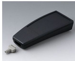
A9068139 SMART-CASE XL, Vers. IV ABS (UL 94 HB) black RAL 9005 168x74,4x35,4mm IP 65 opt., IP 40
