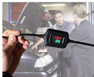
Voltage and current display during trickle charging
