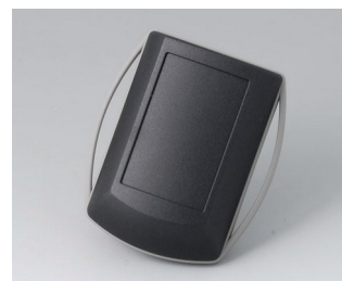
B7040229 ERGO-CASE XS ABS (UL 94 HB) black RAL 9005 82x56x24mm IP 42
