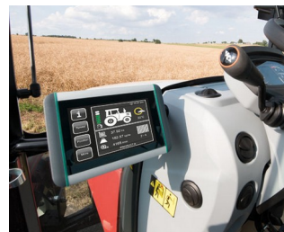
ISOBUS terminal for tractors and self-propelled machines
