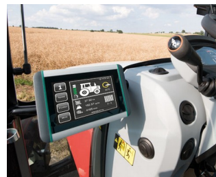
ISOBUS terminal for tractors and self-propelled machines
