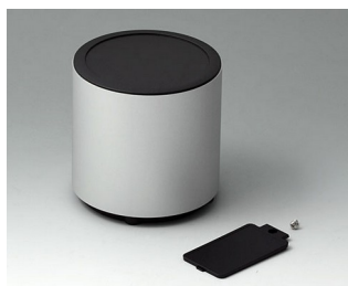
ER109059 SYNERGY R100 Aluminium AlMgSi 0,5 matt anodised ø100x100mm IP 40
