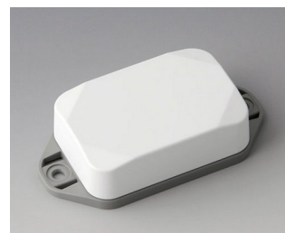
B1822226 MINI-DATA-BOX EF40, high, with flanges ASA+PC (UL 94 V-0) traffic white RAL 9016 60x40x20mm IP 65 opt., IP 40
