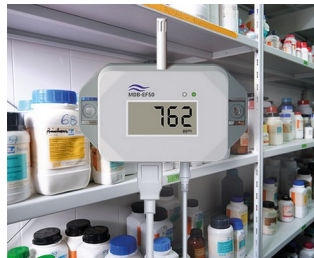
Gas detector for hazardous substances
