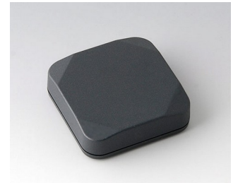
B1804118 MINI-DATA-BOX S50, flat ASA+PC (UL 94 V-0) anthracite grey RAL 7016 50x50x15mm IP 65 opt., IP 40
