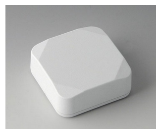
B1804217 MINI-DATA-BOX S50, high ASA+PC (UL 94 V-0) traffic white RAL 9016 50x50x20mm IP 65 opt., IP 40
