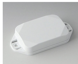
B1822127 MINI-DATA-BOX EF40, flat, with flanges ASA+PC (UL 94 V-0) traffic white RAL 9016 60x40x15mm IP 65 opt., IP 40
