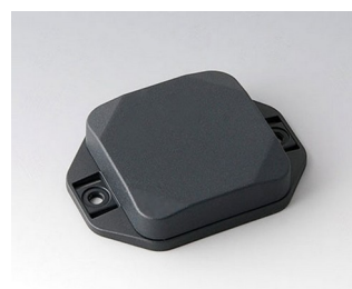
B1804128 MINI-DATA-BOX SF50, flat, with flanges ASA+PC (UL 94 V-0) anthracite grey RAL 7016 50x50x15mm IP 65 opt., IP 40
