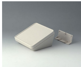
B4414207 PROTEC 140, Vers. II ASA+PC (UL 94 V-0) off-white RAL 9002 140x140x76mm IP 65 opt.
