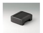
C8011131 SOLID-BOX 115 PC+ABS (UL 94 V-0) anthracite grey RAL 7016 135x115x50mm IP 66, IP 67, IK 08
