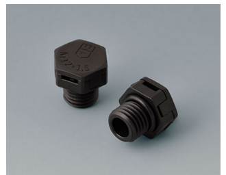
C2305969 Pressure equalisation element M12x1.5 – High-Airflow PA 6 (UL 94 V-0) black RAL 9005
