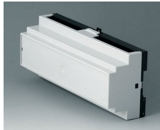
B6506112 RAILTEC B, 12 modules, Vers. II PC (UL 94 V-0) light grey RAL 7035 210x90x58mm
