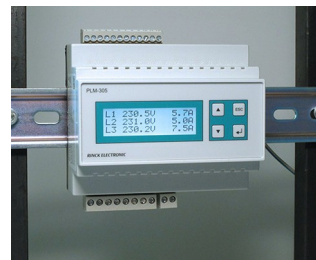
Power measuring device for energy analysis
