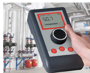
Find compressed air leaks using ultrasound
