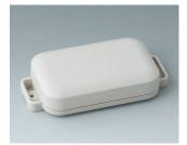
C3206107 EASYTEC 100 ASA+PC (UL 94 V-0) off-white RAL 9002 121x62x26mm IP 65 opt., IP 40
