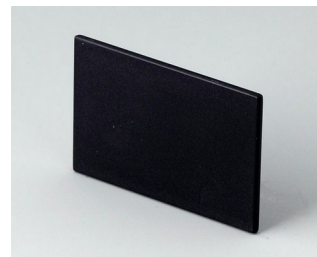
B6112222 Rear panel PPO (UL 94 V-0) black RAL 9005 42,3x29,6x1,8mm
