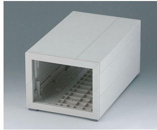
B2212217 MEDITEC E 220, without handle bar ABS (UL 94 HB) off-white RAL 9002 160x260x124mm IP 40
