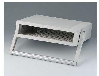
B2210107 MEDITEC D 220, with handle bar ABS (UL 94 HB) off-white RAL 9002 290x260x74mm IP 40
