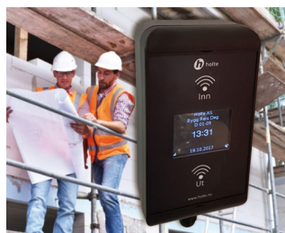
RFID card reader for construction site workers
