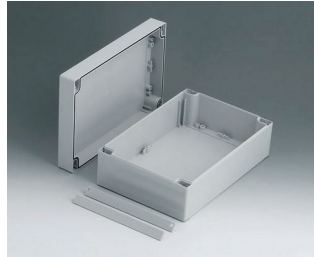
C2116242 ROBUST-BOX WIDTH 160, Vers. II PC (UL 94 HB) light grey RAL 7035 240x160x90mm IP 66
