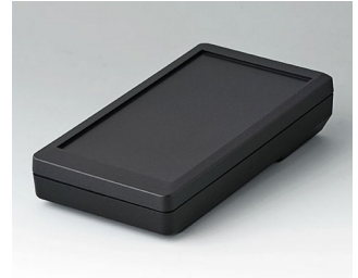
A9073119 DATEC-MOBIL-BOX S, Vers. I ABS (UL 94 HB) black RAL 9005 152x83x33,5mm IP 65 opt.
