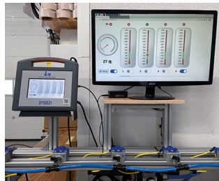
Monitoring system for cleaning nozzles
