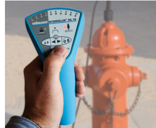
One-handed ground microphone
