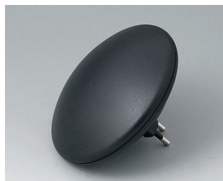
B5011129 ART-CASE R110 H PC+ABS (UL 94 V-0) black RAL 9005 ø110x38mm IP 40
