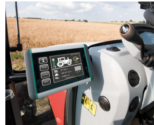
ISOBUS terminal for tractors and self-propelled machines
