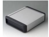
B3407012 SMART-TERMINAL 160 Aluminium AIMgSi 0,5 matt anodised 202x170x50mm IP 54
