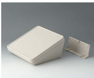
B4418207 PROTEC 180, Vers. II ASA+PC (UL 94 V-0) gris blanc RAL 9002 180x180x92mm IP 65 opt.
