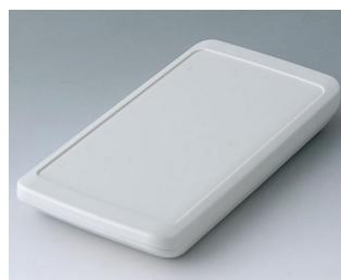
B5403207 SLIM-CASE M, Vers. II ASA+PC (UL 94 V-0) gris blanc RAL 9002 148x74x19mm IP 65 opt., IP 40
