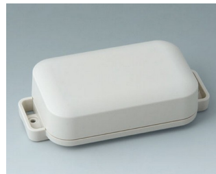
C3206207 EASYTEC 100 ASA+PC (UL 94 V-0) gris blanc RAL 9002 121x62x31mm IP 65 opt., IP 40
