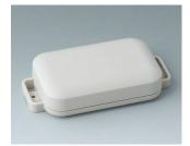
C3206107 EASYTEC 100 ASA+PC (UL 94 V-0) gris blanc RAL 9002 121x62x26mm IP 65 opt., IP 40
