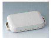
C3207107 EASYTEC 125 ASA+PC (UL 94 V-0) gris blanc RAL 9002 147x78x30mm IP 65 opt., IP 40
