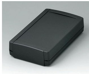
B1075369 TOPTEC 194 F, Vers. I ABS (UL 94 HB) noir RAL 9005 194x115x46mm IP 40
