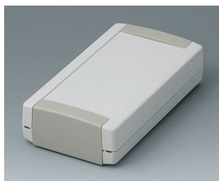
B1065365 TOPTEC 154 F, Vers. I ABS (UL 94 HB) gris blanc RAL 9002 154x84x38mm IP 40
