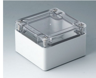
C7008014 IN-BOX ABS/PC (UL 94 HB) gris clair RAL 7035 84x82x55mm IP 66, IP 67, IK 07
