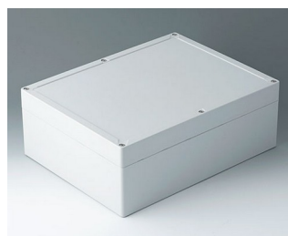
C7030111 IN-BOX ABS (UL 94 HB) gris clair RAL 7035 302x232x110mm IP 66, IP 67, IK 07
