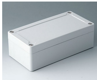
C7016011 IN-BOX ABS (UL 94 HB) gris clair RAL 7035 162x82x55mm IP 66, IP 67, IK 07
