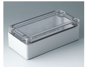
C7016014 IN-BOX ABS/PC (UL 94 HB) gris clair RAL 7035 162x82x55mm IP 66, IP 67, IK 07
