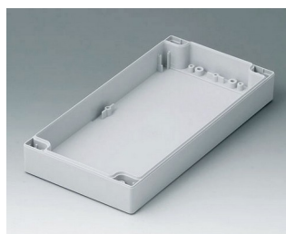
C0122402 Coquille 120, sans joint PC (UL 94 HB) gris clair RAL 7035 240x120x30mm
