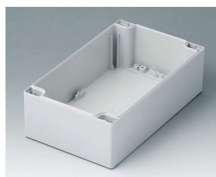
C2122002 Coquille 120, sans joint PC (UL 94 HB) gris clair RAL 7035 200x120x60mm
