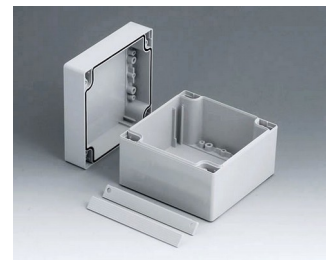
C2112122 ROBUST-BOX 120 LARGE, Vers. II PC (UL 94 HB) gris clair RAL 7035 120x120x90mm IP 66
