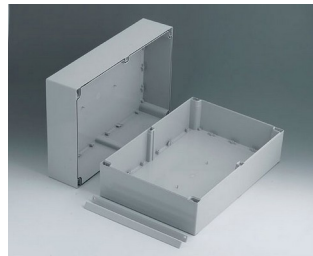
C2524361 ROBUST-BOX 240 LARGE, Vers. I ABS (UL 94 HB) gris clair RAL 7035 360x240x160mm IP 66
