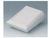
A0612107 COMTEC 120 H, Vers. I ABS (UL 94 HB) gris blanc RAL 9002 120x150x62,8mm IP 40
