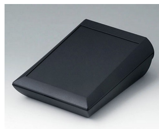
A0615109 COMTEC 150 H, Vers. I ABS (UL 94 HB) noir RAL 9005 150x200x71,5mm IP 40
