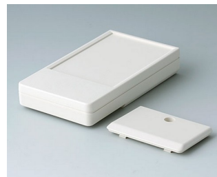
A9071107 DATEC-POCKET-BOX M ABS (UL 94 HB) gris blanc RAL 9002 105x58x18,5mm IP 41
