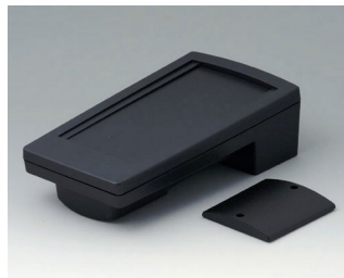
A9046109 HAND-TERMINAL M, Vers. I PC+ABS (UL 94 V-0) noir RAL 9005 220x120x65mm IP 65 opt.
