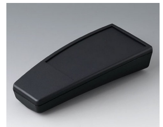
A9068119 SMART-CASE XL, Vers. II ABS (UL 94 HB) noir RAL 9005 168x74,4x35,4mm IP 65 opt., IP 40
