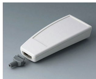
A9067137 SMART-CASE L, Vers. IV ABS (UL 94 HB) gris blanc RAL 9002 140x62,7x30,5mm IP 65 opt., IP 40
