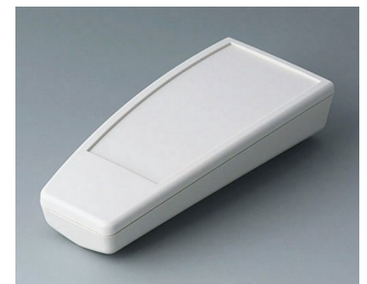
A9067117 SMART-CASE L, Vers. II ABS (UL 94 HB) gris blanc RAL 9002 140x62,7x30,5mm IP 65 opt., IP 40
