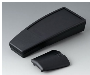
A9068109 SMART-CASE XL, Vers. I ABS (UL 94 HB) noir RAL 9005 168x74,4x35,4mm IP 40
