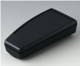
A9066319 SMART-CASE M, Vers. VI ABS (UL 94 HB) noir RAL 9005 96x47x24mm IP 40
