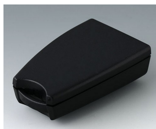
A9064109 SMART-CASE XS ABS (UL 94 HB) noir RAL 9005 58x35,6x19mm IP 40
