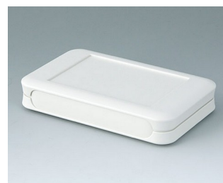
A9051107 SOFT-CASE M ABS (UL 94 HB) gris blanc RAL 9002 65x105x19mm IP 54 opt., IP 40
