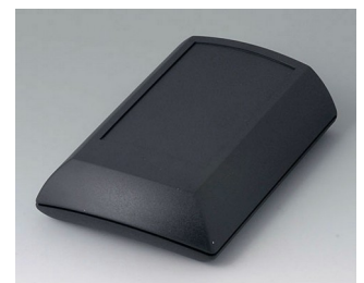
B7010209 ERGO-CASE M, plate ABS (UL 94 HB) noir RAL 9005 150x100x40mm IP 54 opt.
