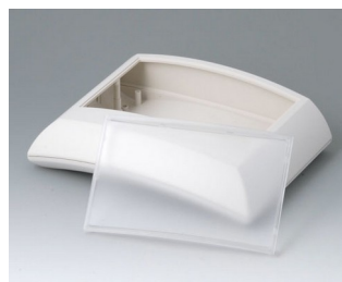
B7020247 ERGO-CASE L, plate ABS (UL 94 HB) gris blanc RAL 9002 150x200x54mm IP 40
