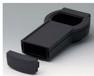
A9078209 DATEC-CONTROL M, Vers. II ABS (UL 94 HB) noir RAL 9005 243x130x60mm IP 54 opt.
