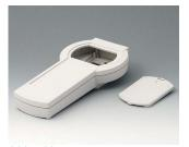
A9077207 DATEC-CONTROL S, Vers. II ABS (UL 94 HB) gris blanc RAL 9002 228x117x47mm IP 65 opt.
