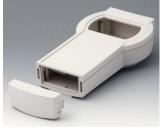
A9078207 DATEC-CONTROL M, Vers. II ABS (UL 94 HB) gris blanc RAL 9002 243x130x60mm IP 54 opt.
