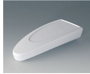
B2804027 STYLE-CASE L ASA (UL 94 HB) blanc signalisation RAL 9016 166x64x31mm IP 65 opt., IP 40
