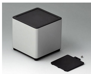
ES109059 SYNERGY S100 Aluminium AIMgSi 0,5 anodisé mat 100x100x100mm IP 40
