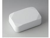
B1822217 MINI-DATA-BOX E40, haute ASA+PC (UL 94 V-0) blanc signalisation RAL 9016 60x40x20mm IP 65 opt., IP 40
