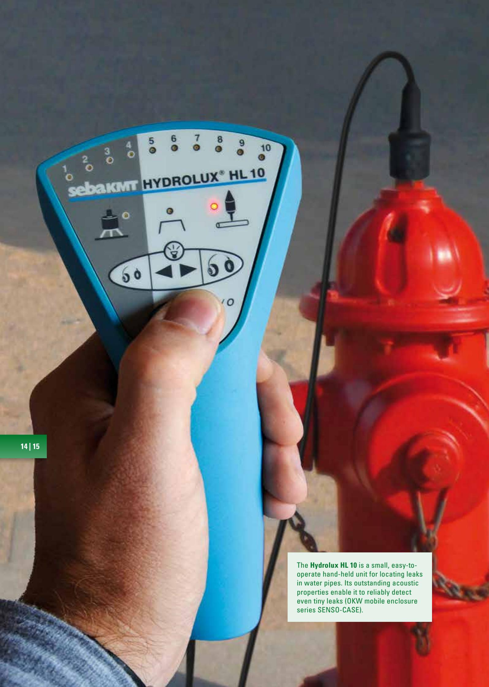
The **Hydrolux HL 10** is a small, easy-to-operate hand-held unit for locating leaks in water pipes. Its outstanding acoustic properties enable it to reliably detect even tiny leaks (OKW mobile enclosure series SENSO-CASE).
