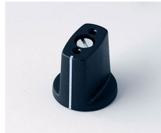
A2416040 SPINDLE-SHAPED KNOB 16, with line ABS (UL 94 HB) black RAL 9005 16x16mm 4mm
