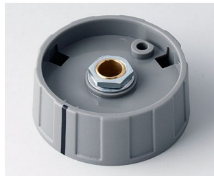
A2640068 ROUND KNOB 40, with line ABS (UL 94 HB) dusty grey RAL 7037 40x15mm 6mm
