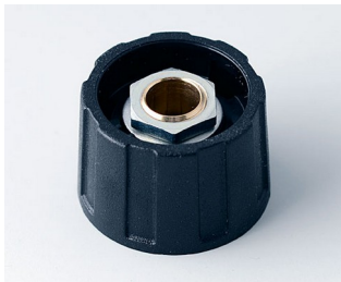
A2523630 ROUND KNOB 23, without line ABS (UL 94 HB) black RAL 9005 23x15mm 1/4"
