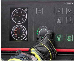
Control element for pump control station
