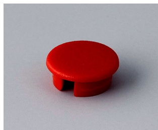
A4110002 Cover 10, without line ABS (UL 94 HB) red RAL F12/0-10
