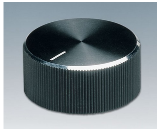
A1432260 TUNING KNOB, with lateral screw fixing ABS (UL 94 HB) black/alu 33x14,3mm 6mm
