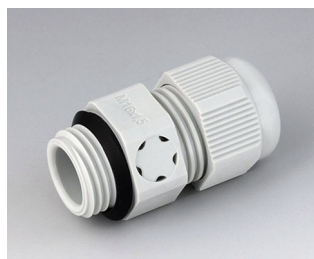
C2316917 Cable gland M16x1.5, pressure compensation PA 6 (UL 94 V-0) light grey RAL 7035
