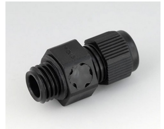
C2312919 Cable gland M12x1.5, pressure compensation PA 6 (UL 94 V-0) black RAL 9005
